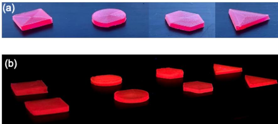
Figure 42: (a) Picture of concentric printed parts under natural sunlight illumination. (b) Picture of concentric (bottom row) and zigzag (top row) printed parts under UV illumination.
