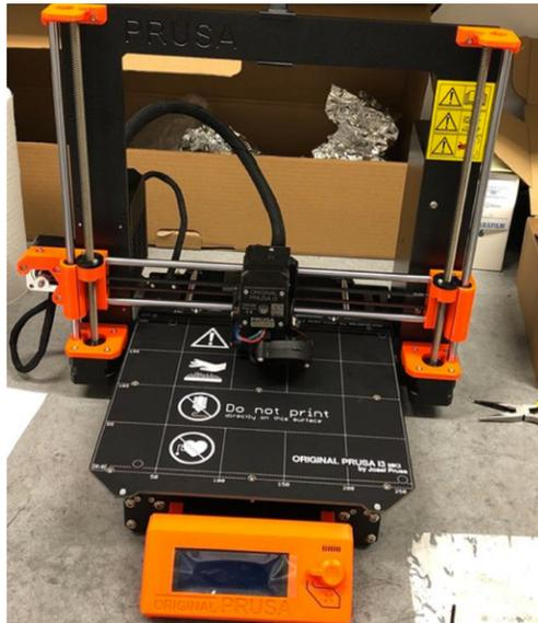
*Figure 26: Photograph of Prusa MK3S printer when first assembled. This is a highly accessible, commercially available printer with modification capabilities.*
