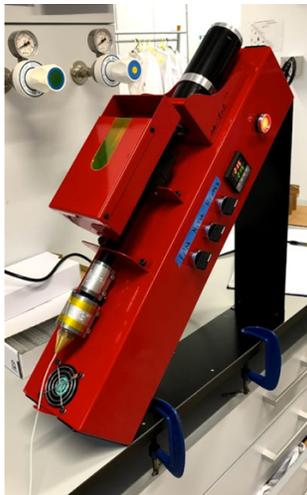
*Figure 25: Photograph of Noztek Pro Filament Extruder used in this study. Shows the motor, heater, hopper, and dials used to control the extruder. Test, non-luminescent ABS filament is being produced in this picture.*
