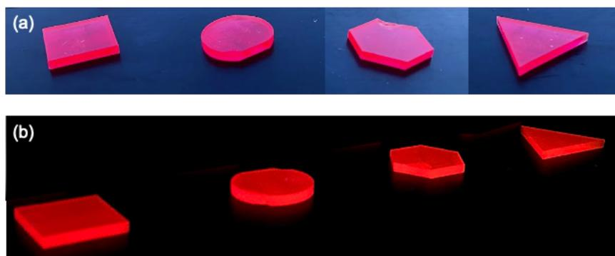
Figure 43: (a) Picture of laser cut PMMA + LR305 LSC under natural sunlight illumination. (b) Picture of laser cut LSCs under UV illumination.
